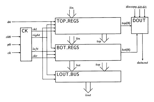
Figure 9.3: Implementation of the SHIFTREGS Device
