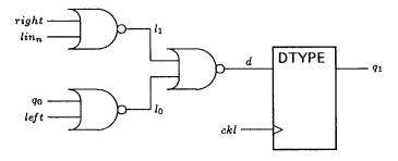
Figure 9.5: Implementation of a Register Cell
