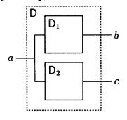
The structure of such a device can be specified using the and construct in a let statement which allows simultaneous declarations. This neatly captures the notion of devices connected in parallel where the values on the output lines are calculated as function applications of the input lines independent of one device to another. The order in which the output values are calculated in a simultaneous declaration is irrelevant.
