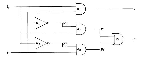
Figure 4.3: Implementation of a Half-Adder
