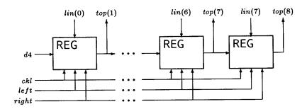
Figure 9.4: Implementation of a Shift Register
