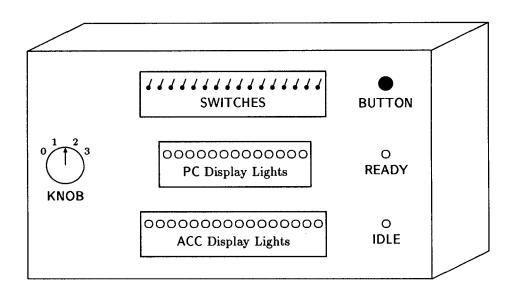
Figure 8.1: Front Panel of Gordon's Computer
