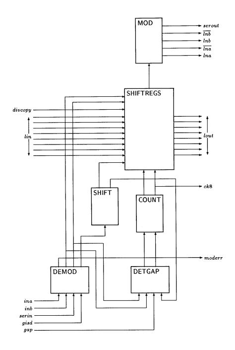
Figure 9.2: Top-level Implementation of ECL Chip
