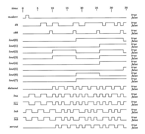
Figure 9.7: Waveforms Showing Outputs from ECL Chip
