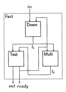
Figure 7.2: Implementation of Factorial Device
