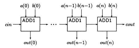
Figure 3.4: Implementation of a Binary Adder
