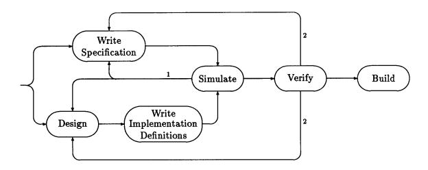
Figure 1.1: The Ideal Verification Process
