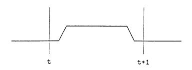
Figure 10: A Signal which is Not "Well-Behaved"
