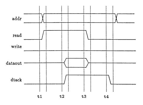
Figure 4: Read Cycle using a Four-Phase Handshaking Protocol. This simplified timing diagram shows the relative order of events in a read cycle where a request occurs at t1 followed by an acknowledgement at t2. The acknowledgement may occur in the same interval as the request, i.e. t2 may be equal to t1. Similarly, t4 may be equal to t3. However, t3 must occur strictly after t1 and t4 strictly after t2 since signals are not allowed to rise and fall within the same interval.
