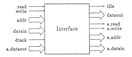
Figure 5: Synchronous Interface Device
