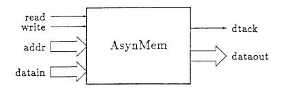
Figure 3: Asynchronous Memory Device
