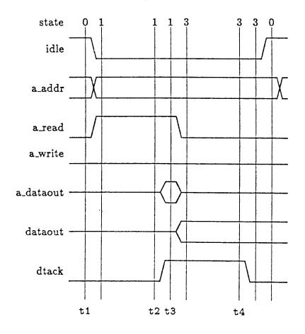
Figure 7: Interaction of State Machine with Asynchronous Memory
