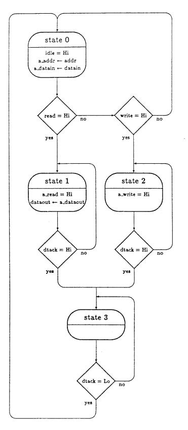
Figure 6: Flow Graph for the Synchronous Interface
