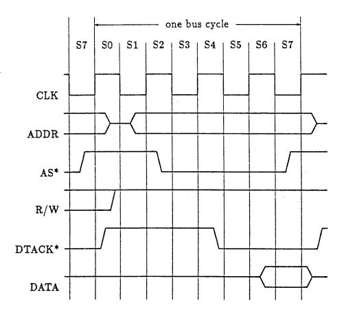
Figure 12: Simplified M68000 Read Cycle. The synchronous time scale for the M68000 is divided into half cycle intervals because events can occur on both rising and falling edges. Only the address strobe AS\* is mentioned here. Asterisks indicate "active-low" signals. This timing diagram is adapted from [2], page 121.
