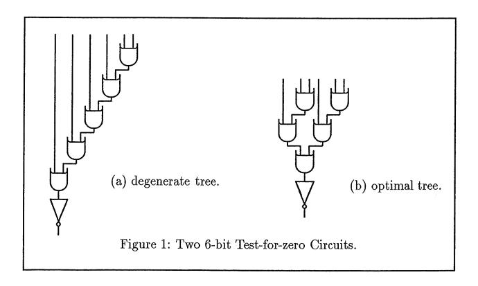
an 'executable' function which generates a provably optimal implementation for any input width.
