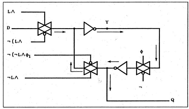
Figure 3: A CMOS Dynamic Latch with Signal Flow
