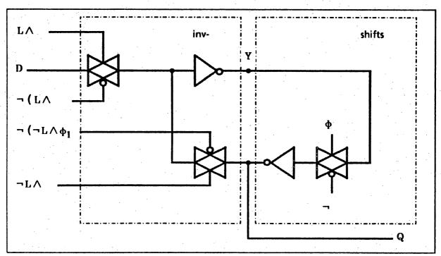
Figure 2: A CMOS Dynamic Latch
