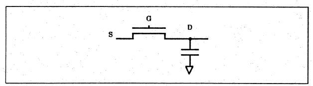
Figure 7: A Pass Transistor with Explicit Capacitance
