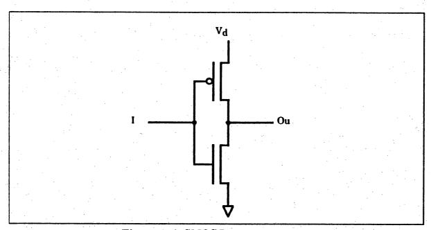
Figure 1: A CMOS Inverter
