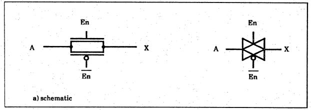
Figure 6: A CMOS Transmission Gate
