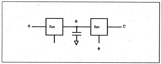
Figure 10: An Element which Employs 2-phase Clocking
