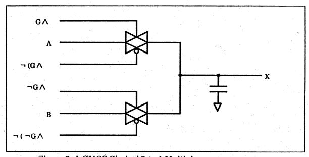
Figure 9: A CMOS Clocked 2-to-1 Multiplexer
