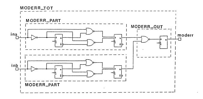
Figure 5: Modulation Error Detector
