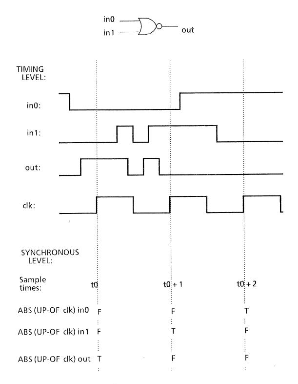
Figure 2: Temporal abstraction of timing level NOR signals
