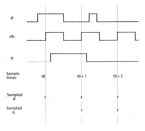
Figure 1: Sampling of flip-flop signals
