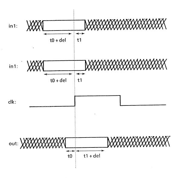
Figure 3: Stability relationship for timing level NOR signals
