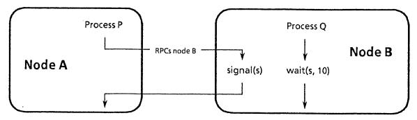
Figure 2. Breakpointing with remote processes.
