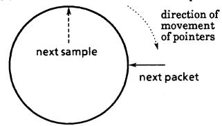
Position of the pointers with first packet received, after waiting time j. For convenience, these diagrams are drawn for d=j. In these figures, next sample is used as reference and is always shown in the same position.
