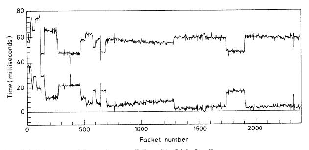
Figure 2.4: Adjustment of Excess Reserve, Followed by Light Loading
