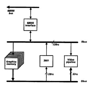
Figure 9.1. The display's bus structure
