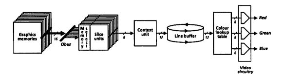
Figure 8.1. Video generation pipeline
