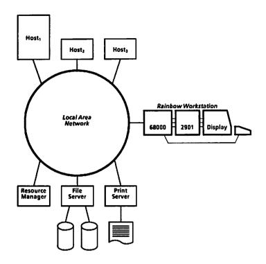
Figure 7.1. The Rainbow Workstation in the Cambridge Distributed System
