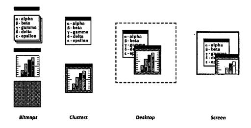
Figure 10.3. Mapping bitmaps onto the screen
