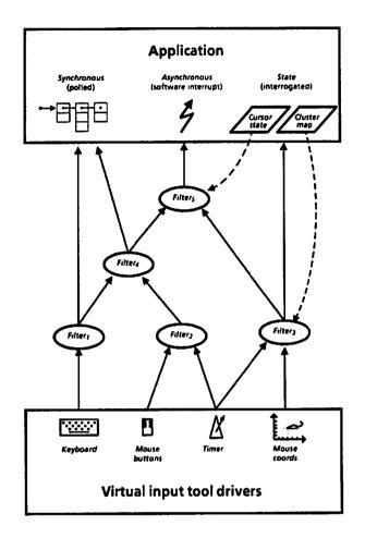
Figure 10.4. The input tool scheme
