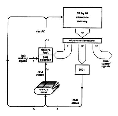
Figure 9.2. The microcode instruction pipeline
