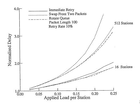
Figure 6.6: Delay at Low Loads using Queue Manipulation
