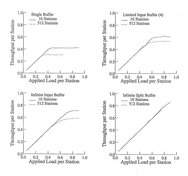
Figure 6.2: Throughput vs. Applied Load: Buffered Network
