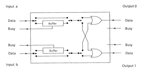
Figure 4.1: Binary Routing Node
