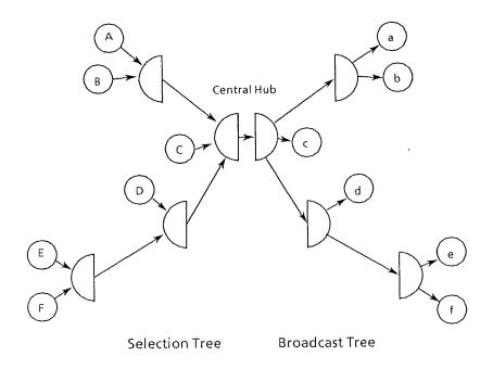
Figure 2.4: Hubnet:Expanded to show Selection and Broadcast Trees
