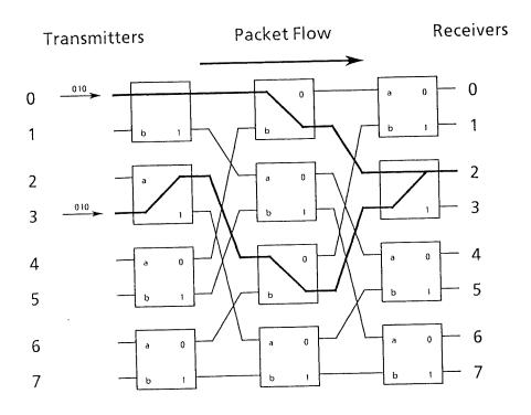
Figure 5.2: Path Equivalence in an Omega Network
