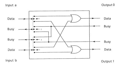
Figure 5.1: Basic Structure of Non-Buffered Routing Node
