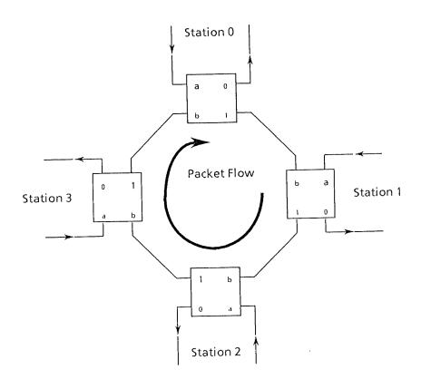
Figure 4.3: BRN Connected as Ring
