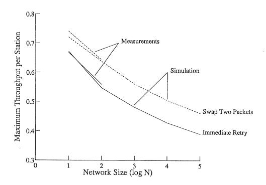
Figure 7.7: Comparison of Simulation and Measurement Results
