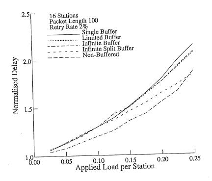
Figure 6.9: Normalised Delay at Low Loads: 16 Stations
