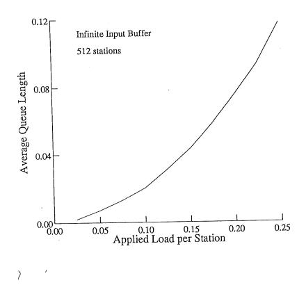
Figure 6.12: Average Node Queue Length for a Buffered Network
