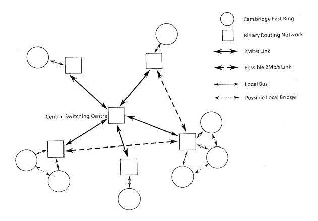
Figure 8.1: Possible Unison Structure using a Binary Routing Network
