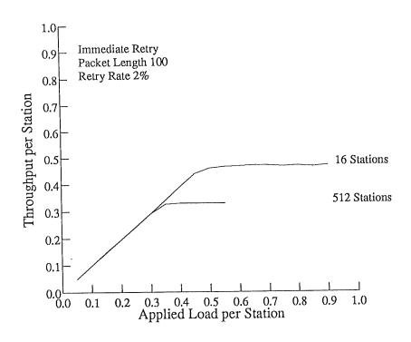
Figure 6.3: Throughput vs. Applied Load: Non-Buffered Network
