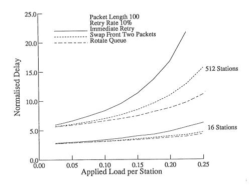
Figure 6.7: Delay for Burst Mode Operation and Queue Manipulation
