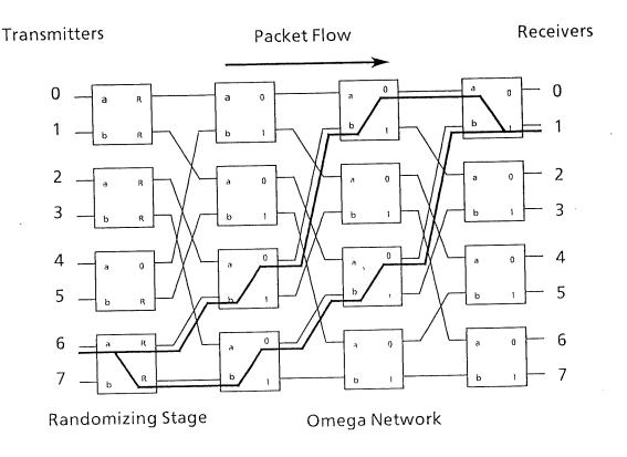
Figure 5.3: BRN with Redundant Paths
