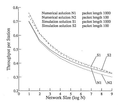
Figure 6.14: Numeric and Simulation Values for the maximum throughput of Non-Buffered BRNs
