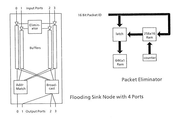
Figure 2.6: A Flooding Sink Switching Node
