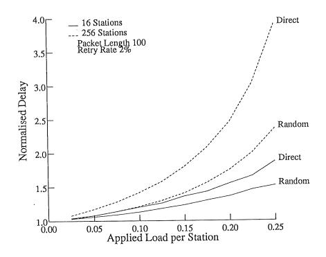
Figure 6.8: Delay of Non-Buffered Networks with and without Random Routing
