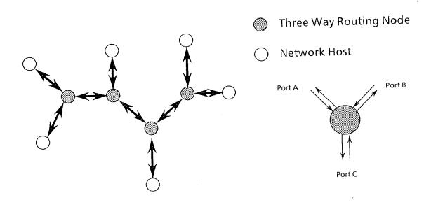
Figure 4.6: BRN Constructed from Three Way Nodes
