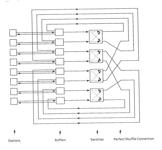
Figure 3.3: Single Stage Shuffle Exchange Network
