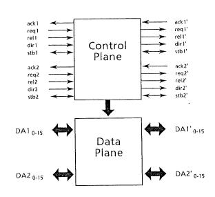
Figure 3.6: Starnet Switching Node
