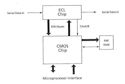
Figure 2.5: Cambridge Fast Ring: ECL and CMOS chip Interconnections
