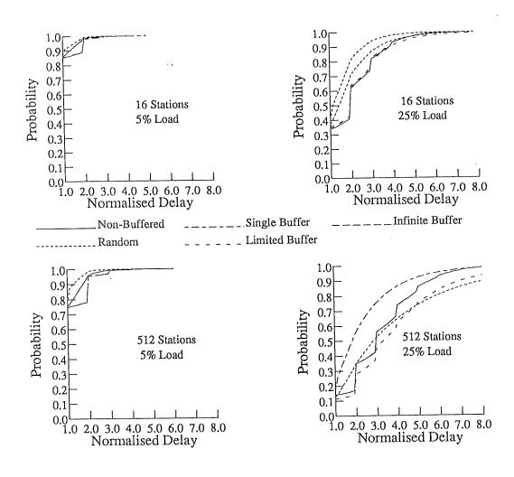
Figure 6.11: Cumulative Probability Functions for Packet Delays
