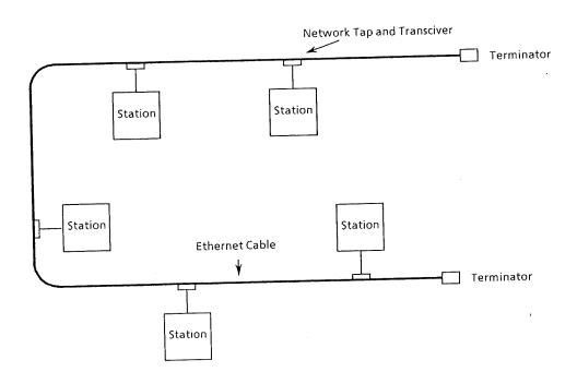
Figure 2.1: Structure of Ethernet
