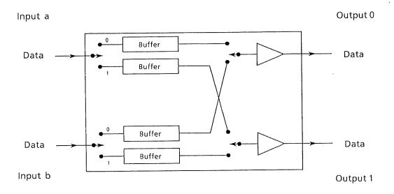
Figure 4.7: Routing Node with Split Buffer Scheme
