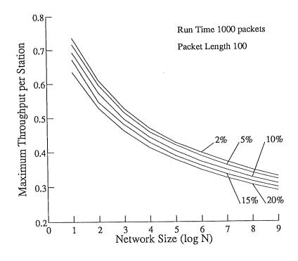
Figure 6.4: Maximum Throughput vs. Network Size for different retry rates: Non-Buffered Network with Immediate Retry
