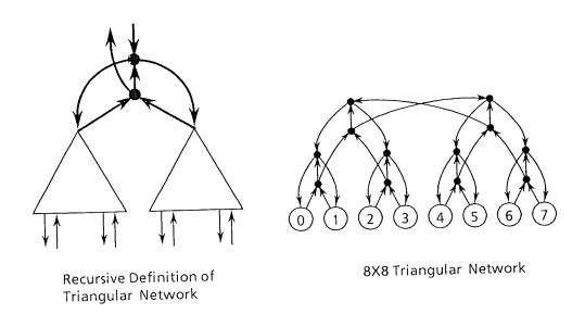
Figure 4.4: A Triangular Network Structure
