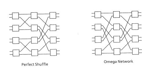
Figure 3.5: Alternative Network Structures
