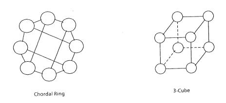
Figure 3.1: Some Static Interconnection Structures
