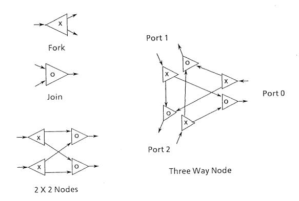
Figure 4.2: Routing Nodes constructed from Fork and Join Units
