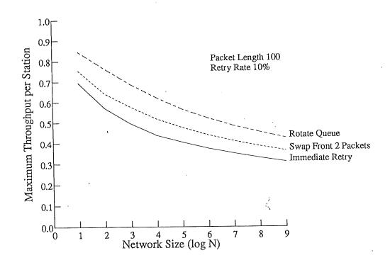
Figure 6.5: Maximum Throughput using Queue Manipulation
