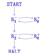
**Claim:** starting from initial configuration (0, 0, x, y), this machine's computation halts with configuration (4, x + y, 0, 0).
