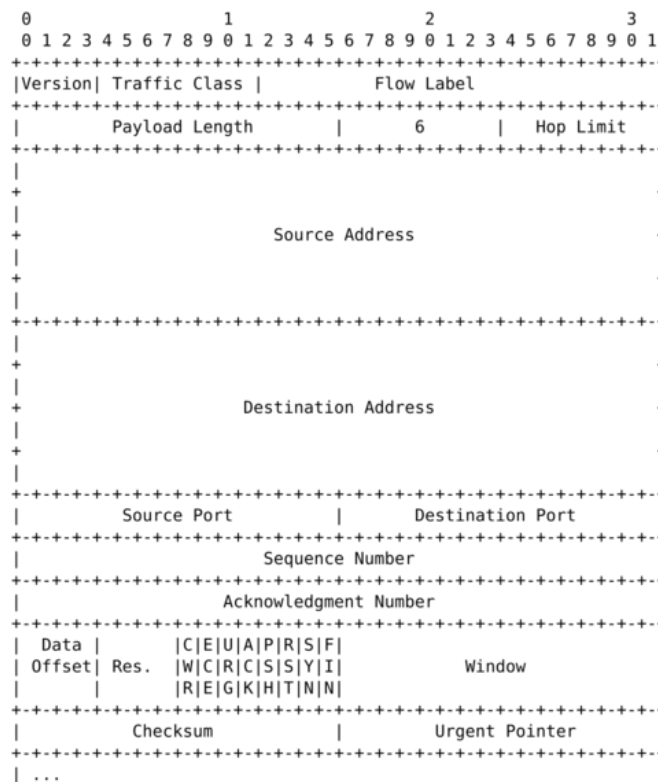
Fig. 45: An IPv6 packet containing an TCP segment
