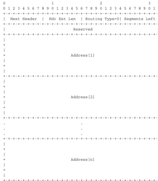
Fig. 50: The Type 0 routing header ( RFC 2460 )
