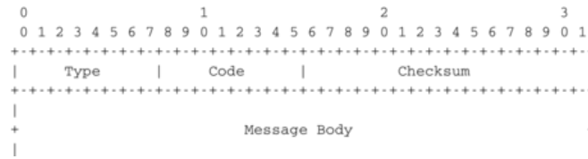
Fig. 51: ICMP version 6 packet format
