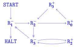
If the machine is started with  $(R_0, R_1, R_2, R_3) = (0, x, y, 0)$ , it halts with  $(R_0, R_1, R_2, R_3) = (xy, 0, y, 0)$ .
