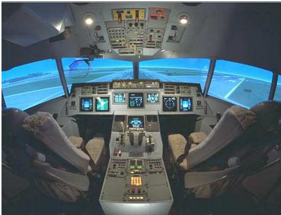
Figure 10: The real cockpit of a commercial flight simulator: an exact replica of the equivalent airplane's cockpit.
