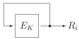
Again, the key K should be replaced before in the order of  $2^{\frac{n}{2}}$  n-bit blocks have been generated, otherwise the random block generator is likely to enter a cycle where  $R_i = R_{i-k}$  for some k in the order of  $2^{\frac{n}{2}}$ .
