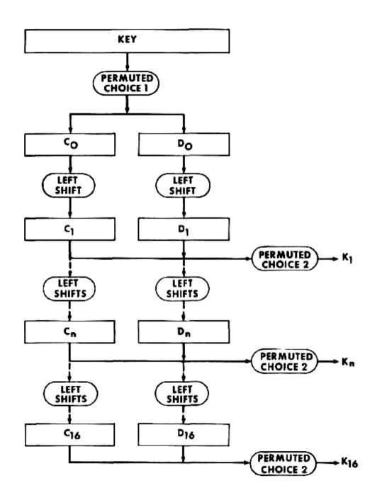
The key schedule of DES breaks the key into two 28-bit halves, which are left shifted by two bits in most rounds (only one bit in round 1,2,9,16) before 48-bit are selected as the subkey for each round.
