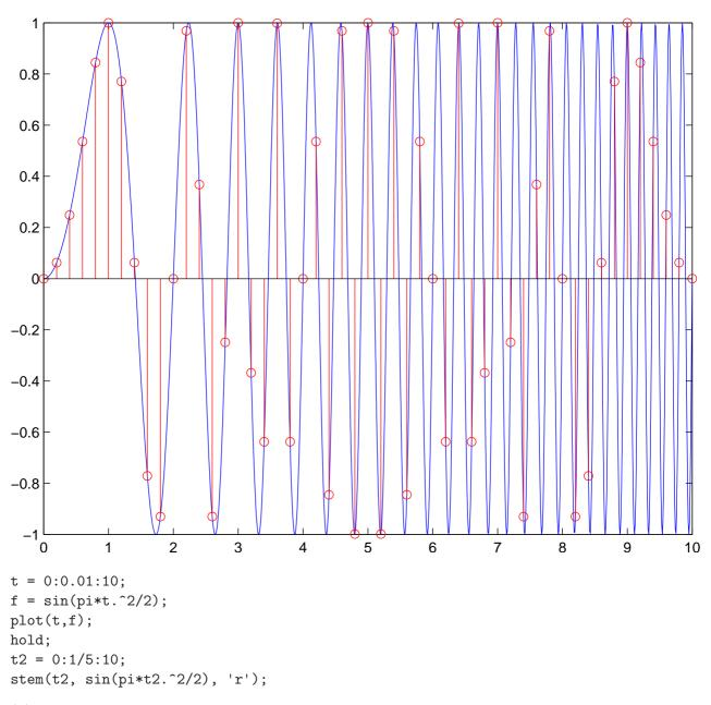
(d) A sine wave with a frequency f larger than half the sampling frequency  $f_s$  cannot be distinguished based on the sample values from a sine wave of frequency  $f_s - f$ . In other words, the sample values would have looked the same had we replaced the instantaneous frequency f(t) with  $f_s/2 - |f_s/2 - f(t)|$ , and the latter is symmetric around  $f_s/2$ , which is in this graph 2.5 Hz and occurs at t = 5 s.
