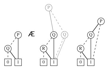
The new construction is shown in grey. In both of these examples, it appears over the rightmost formula because its variables come later in the ordering.
