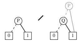
The BDD for  $Q \vee R$  has a similar construction, so we omit it. We combine the two small BDDs using  $\rightarrow$ , then simplify (removing a redundant test on Q) to obtain the final BDD.
