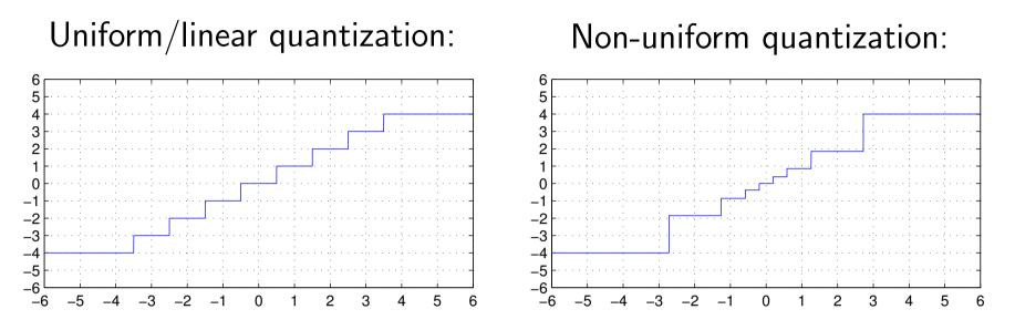
Quantization is the mapping from a continuous or large set of values (e.g., analog voltage, floating-point number) to a smaller set of (typically  $2^8$ ,  $2^{12}$  or  $2^{16}$ ) values.
