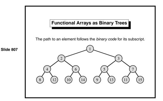
This simple representation (credited to W. Braun) ensures that the tree is balanced. Complexity of access is always  $O(\log n)$ , which is optimal. For actual running time, access to conventional arrays is much faster: it requires only a few hardware instructions. Array access is often taken to be O(1), which (as always) presumes that hardware limits are never exceeded.
