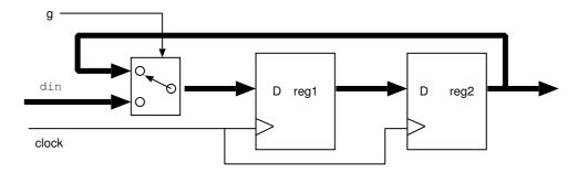
We swap the values between a pair of registers if the guard is false, but a broadside multiplexor introduces a new value into the loop when the guard is enabled.
