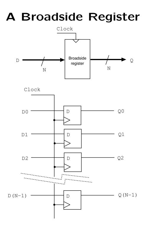
A broadside register of N bits is made out of N D-types with a commoned clock input. It can hold  $2^N$  different values.
