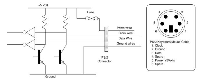
Open collector wiring using two signalling wires.
