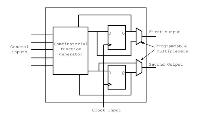
This CLB contains one LUT and two D-type's. The output can be sequential or combinational.
