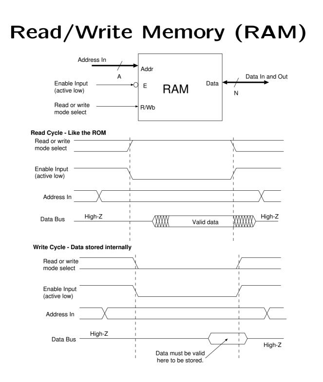
Each data bit internally stored in an RS latch.
