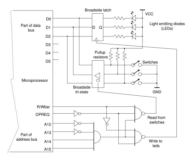
Example of memory address decode and simple LED and switch interfacing for programmed IO (PIO) to a microprocessor.
