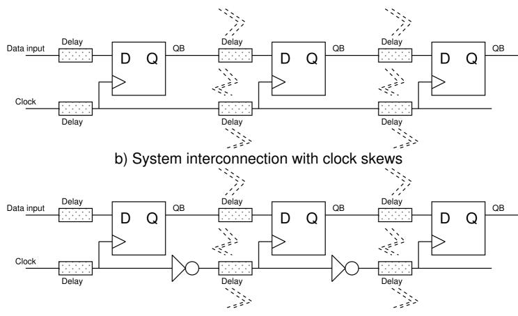
c) A solution for serious skew and delay problems ?
