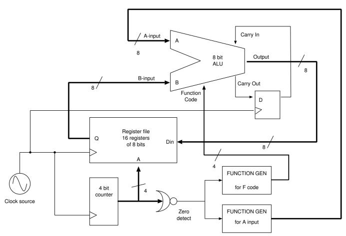
An example structure using an ALU and register file.
