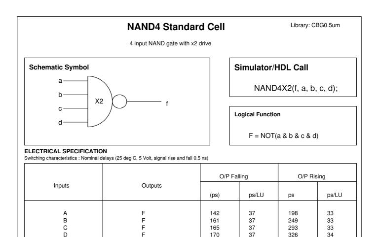
Min and Max delays depend upon temperature range, supply voltage, input edge speed and process spreads. The timing information is for guidance only. Accurate delays are used by the UDC.
