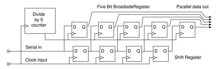
An example that uses (badly) a derived clock: a serial-to-parallel converter
