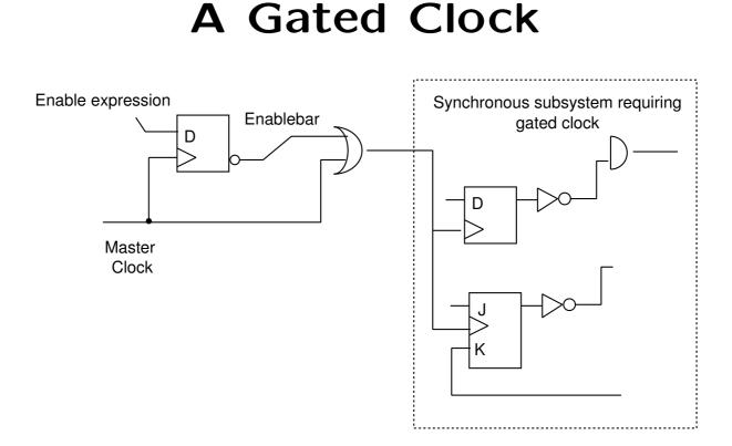
OR'ing with a negated enable works cleanly.
