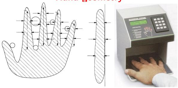
Biometric characteristic used are several dozen length and thicknesses measurements of the fingers. Digital camera captures two hand silhouettes.
