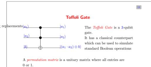
Any  $2^n \times 2^n$  permutation matrix can be implemented using only Toffoli gates.
