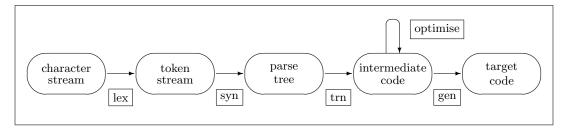
This course only considers the optimiser, which in principle is both source-language and target-architecture independent, but certain gross target features may be exploited (e.g. number of user allocatable registers for a register allocation phase).
