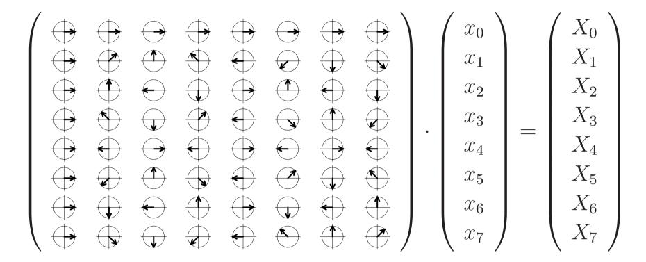
The n-point DFT of a signal  $\{x_i\}$  sampled at frequency  $f_s$  contains in the elements  $X_0$  to  $X_{n/2}$  of the resulting frequency-domain vector the frequency components 0,  $f_s/n$ ,  $2f_s/n$ ,  $3f_s/n$ , ...,  $f_s/2$ , and contains in  $X_{n-1}$  downto  $X_{n/2}$  the corresponding negative frequencies. Note that for a real-valued input vector, both  $X_0$  and  $X_{n/2}$  will be real, too.
