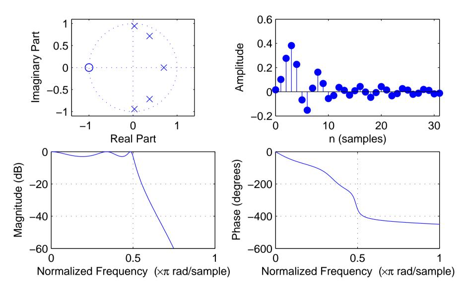
order: 5, cutoff frequency:  $0.5 \times f_{\rm s}/2$ , pass-band ripple:  $-3~{\rm dB}$
