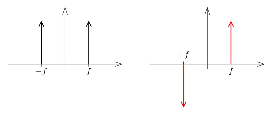
As any real-valued signal x(t) can be represented as a combination of sine and cosine functions, the spectrum of any real-valued signal will show the symmetry  $X(e^{\mathrm{j}\omega}) = [X(e^{-\mathrm{j}\omega})]^*$ , where \* denotes the complex conjugate (i.e., negated imaginary part).
