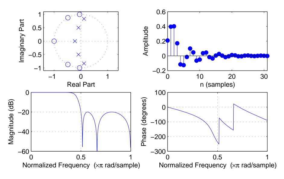
order: 5, cutoff frequency:  $0.5 \times f_{\rm s}/2$ , stop-band ripple:  $-20~{\rm dB}$
