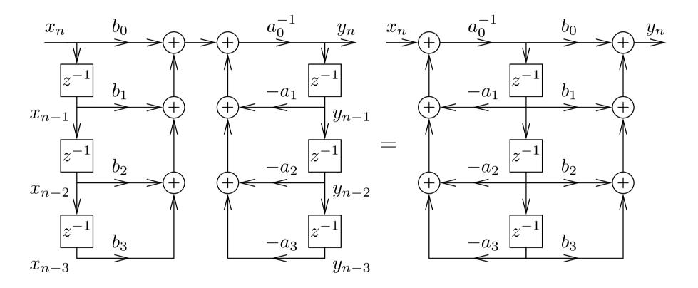
The block diagram representation of the constant-coefficient difference equation on slide 11 is called the *direct form I implementation*. The number of delay elements can be halved by using the commutativity of convolution to swap the two feedback loops, leading to the *direct form II implementation* of the same LTI system.
