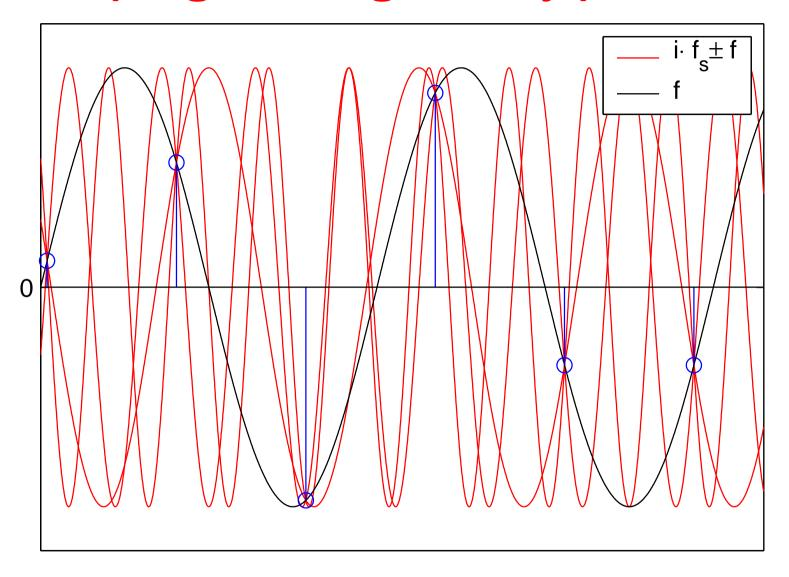
A wave  $\cos(2\pi t f)$  sampled at frequency  $f_s$  cannot be distinguished from  $\cos(2\pi t (k f_s \pm f))$  for any  $k \in \mathbb{Z}$ , therefore ensure  $|f| < f_s/2$ .
