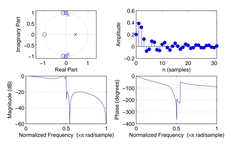
order: 5, cutoff frequency:  $0.5 \times f_{\rm s}/2$ , pass-band ripple: -3 dB, stop-band ripple: -20 dB
