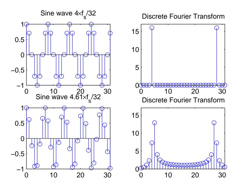
We introduced the DFT as a special case of the continuous Fourier transform, where the input is sampled and periodic.
