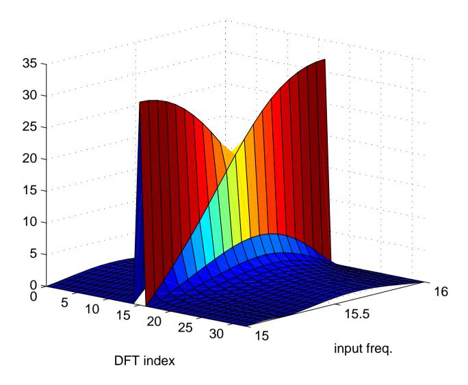
The *leakage* of energy to other frequency bins not only blurs the estimated spectrum. The peak amplitude also changes significantly as the frequency of a tone changes from that associates with one output bin to the next, a phenomenon known as *scalloping*. In the above graphic, an input sine wave gradually changes from the frequency of bin 15 to that of bin 16 (only positive frequencies shown).
