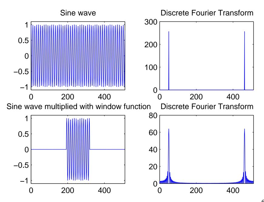
The reason for the leakage and scalloping losses is easy to visualize with the help of the convolution theorem:
