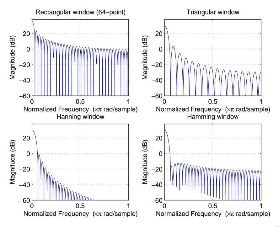
Numerous alternatives to the rectangular window have been proposed that reduce leakage and scalloping in spectral estimation. These are vectors multiplied element-wise with the input vector before applying the DFT to it. They all force the signal amplitude smoothly down to zero at the edge of the window, thereby avoiding the introduction of sharp jumps in the signal when it is extended periodically by the DFT. Three examples of such window vectors  $\{w_i\}_{i=0}^{n-1}$  are:
