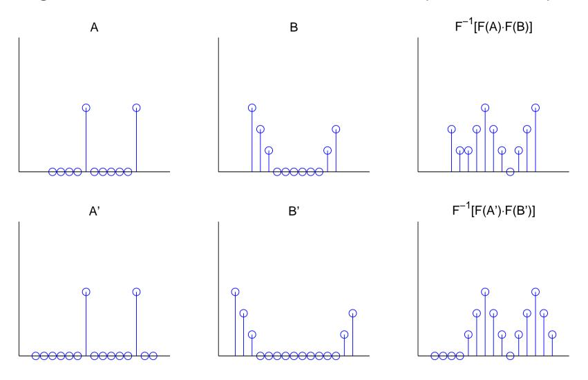
Both sequences are padded by appending zero values to a length of at least m+n-1, to ensure that the start and end of the resulting sequence to not overlap.
