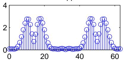
Applying the discrete Fourier transform to an n-element long real-valued sequence leads to a spectrum consisting of only n/2+1 discrete frequencies.
