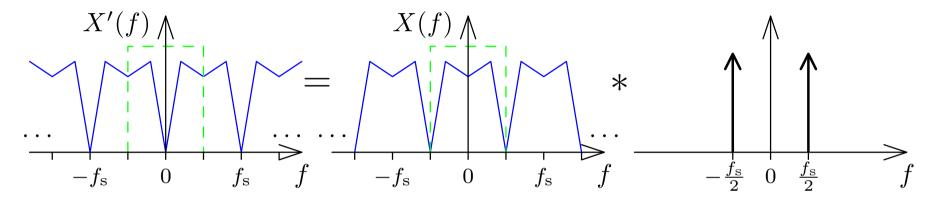
This can be accomplished by multiplying the sampled sequence  $x_i$  with  $y_i = \cos \pi f_s t = \cos \pi i$ , which is nothing but multiplication with the sequence
