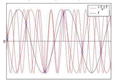
A wave  $\cos(2\pi tf)$  sampled at frequency  $f_{\rm s}$  cannot be distinguished from  $\cos(2\pi t(kf_{\rm s}\pm f))$  for any  $k\in\mathbb{Z}$ , therefore ensure  $|f|< f_s/2$ .
