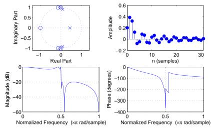
order: 5, cutoff frequency:  $0.5\times f_{\rm s}/2$ , pass-band ripple: -3 dB, stop-band ripple: -20 dB 59
