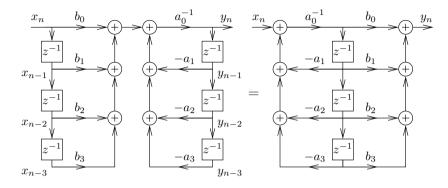
The block diagram representation of the constant-coefficient difference equation on slide 11 is called the *direct form I implementation*. The number of delay elements can be halved by using the commutativity of convolution to swap the two feedback loops, leading to the *direct form II implementation* of the same LTI system.
