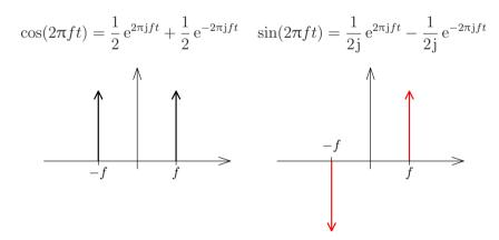
As any real-valued signal x(t) can be represented as a combination of sine and cosine functions, the spectrum of any real-valued signal will show the symmetry  $X(e^{j\omega}) = [X(e^{-j\omega})]^*$ , where \* denotes the complex conjugate (i.e., negated imaginary part).
