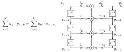
The MATLAB function filter is an efficient implementation of the last variant.
