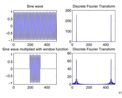
The reason for the leakage and scalloping losses is easy to visualize with the help of the convolution theorem:
