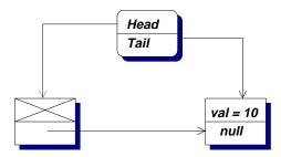
Both of the pop operations would have to return the 10 node if invoked at this time. There will need to be some arbitration between them – either by holding both of the locks at once (note the possibility of deadlock if they can be acquired in any order) or the use of a multi-word atomic operation (see Detlefs *et al*'s work on double-ended queues using DCAS).
