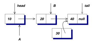
One thread is about to delete the 20 node by performing a CAS at A, changing it from the 20 node to the 40 node. Another thread is about to insert the 30 node by performing a CAS at B, changing it from the 40 node to the 30 node. Both can succeed, leaving this non-linearizable mess:
