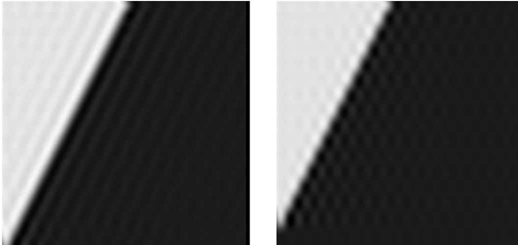
Figure 8: The two images of figure 6 reconstructed using as near perfect reconstruction as possible. (a) on the left and (b) on the right. This figure shows part of the reconstructed intensity surface. Aliasing artifacts occur in (b) only
