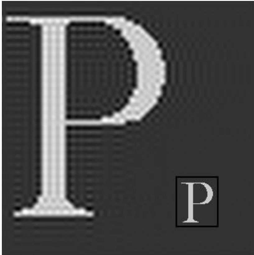
Figure 4: An example of a reconstructed intensity surface which contains aliases. These manifest themselves as ripples around the sharp edges in the image. The small image of the letter 'P' is the original. The large is an intensity surface reconstructed from this small original using an approximation to sinc reconstruction.
