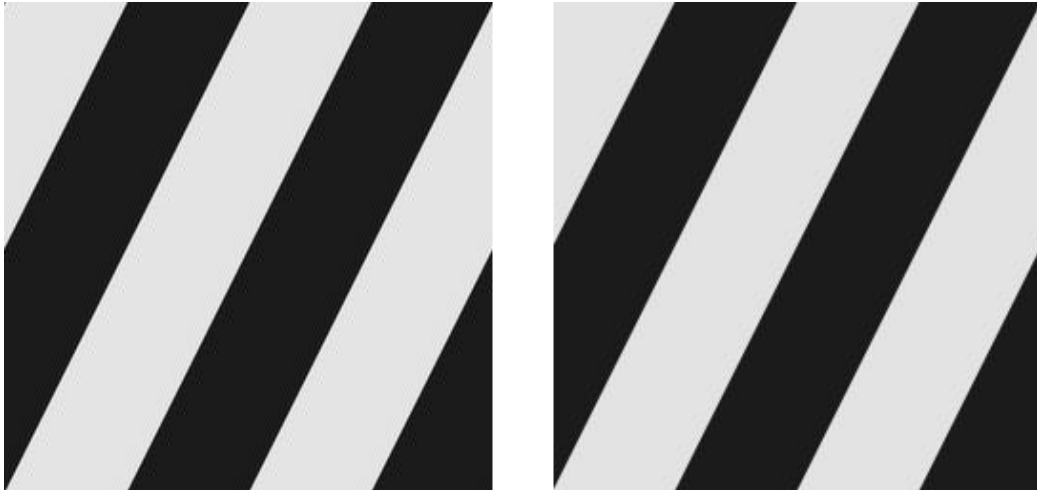
Figure 6: Two very similar images: (a) on the left, was generated by summing the first twenty-nine terms of the Fourier series representation of the appropriate square wave; (b) on the right, was generated by super-sampling a perfect representation of the stripes.
