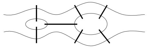
Is it possible to set out from any point in the town and cross each bridge exactly once, returning to the starting point? In this case the answer is "no".
