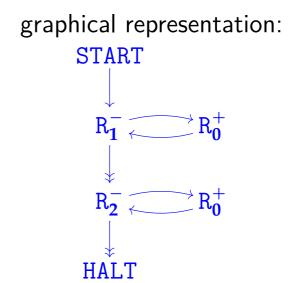
**Claim:** starting from initial configuration (0, 0, x, y), this machine's computation halts with configuration (4, x + y, 0, 0).
