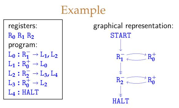
**Claim:** starting from initial configuration (0, 0, x, y), this machine's computation halts with configuration (4, x + y, 0, 0). So  $f(x, y) \triangleq x + y$  is computable.
