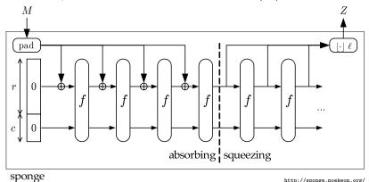
sponge (r+c)-bit internal state, XOR \$r\$-bit input blocks at a time, stir with pseudo-random permutation \$f\$, output \$r\$-bit output blocks at a time.
