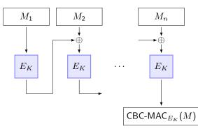
Similar to CBC:  $IV = 0^m$ , last ciphertext block serves as tag. Provides existential unforgeability, but only for **fixed** message length n: Adversary asks oracle for  $T^1 := \text{CBC-MAC}_{E_K}(M^1) = E_K(M^1)$  and then presents  $M = M^1 || (T^1 \oplus M^1)$  and  $T := \text{CBC-MAC}_{E_K}(M) =$  $E_K((M^1 \oplus T^1) \oplus E_K(M^1)) = E_K((M^1 \oplus T^1) \oplus T^1) = E_K(M^1) = T^1.$
