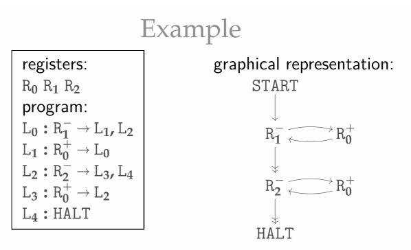
**Claim:** starting from initial configuration (0, 0, x, y), this machine's computation halts with configuration (4, x + y, 0, 0).
