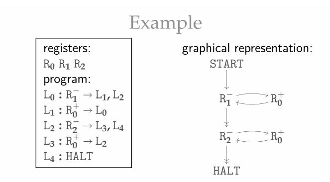
**Claim:** starting from initial configuration (0, 0, x, y), this machine's computation halts with configuration (4, x + y, 0, 0). So  $f(x, y) \triangleq x + y$  is computable.
