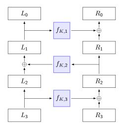
Decryption works backwards, undoing round after round, starting from the ciphertext. This is possible, because the Feistel structure is arranged such that during decryption in any round i = r, ..., 1, the input value for  $f_{K,i}$  is known, as it formed half of all bits of the result of round i during encryption:
