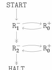
**Claim:** starting from initial configuration (0, 0, x, y), this machine's computation halts with configuration (4, x + y, 0, 0)
