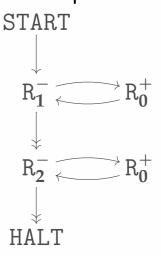
**Claim:** starting from initial configuration (0, 0, x, y), this machine's computation halts with configuration (4, x + y, 0, 0). So  $f(x, y) \triangleq x + y$  is computable.
