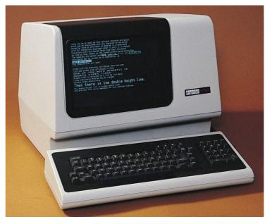
The VT100 was the first video terminal with microprocessor, and the first to implement the ANSI X3.64 (= ECMA-48) control functions. For instance, " $^{E}S_{C}$ [7m" activates inverse mode and " $^{E}S_{C}$ [0m" returns to normal, where  $^{E}S_{C}$  is the ASCII control character encoded by byte 27.
