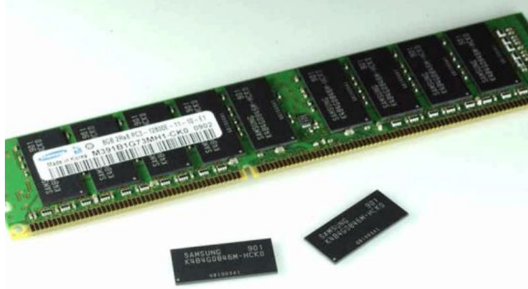
Figure 12.8: DRAM single-in-line memory module (SIMM).
