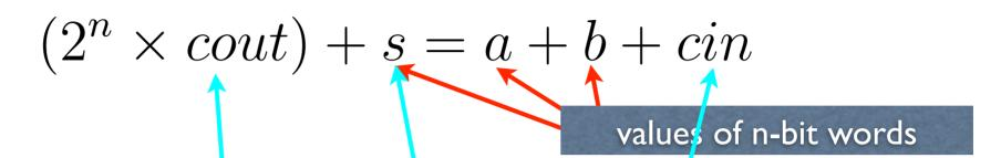
The function bits\_val converts a binary numeral (supplied in the form of a boolean valued function, f) to a non-negative integer. The specification of the adder then follows the obvious arithmetic specification closely. When n=0, the specification merely requires cin=cout.
