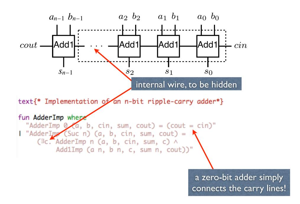
An (n+1)-bit adder consists of a full adder connected to an n-bit adder. Note that AdderImp n specifies an n-bit adder, and in particular, a 0-bit adder is nothing but a wire connecting carry in to carry out.
