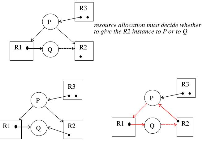
give the R2 instance to Q: no cycle AFAIK, Q can complete and release R1 and R2, then P can have R1 and R2 and complete. There may of course be further dynamic requests.
