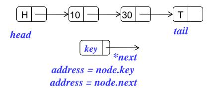
Insertion is straightforward. First, the list is traversed until the correct position is found. Then a new cell is created and inserted using *CAS* (compare and swap)
