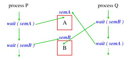
At this point we have deadlock. Process P holds *semA* and is blocked, queued on *semB*Process Q holds *semB* and is blocked, queued on *semA*Neither process can proceed to use the resources and signal the respective semaphores.
