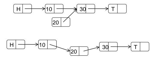
*CAS* (*address*, *old*, *new*) atomically compares the contents of *address* with the *old* value and, if they match, writes the *new* value to that location.
