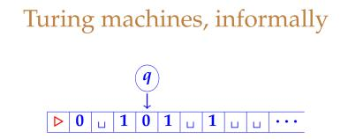
► Machine starts with tape head pointing to the special left endmarker ▷.
