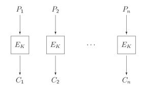
In the simplest **mode of operation** standardised for DES, AES, and other block ciphers, the message is cut into n-bit blocks, where n is the block size of the cipher, and then the cipher function is applied to each block individually.
