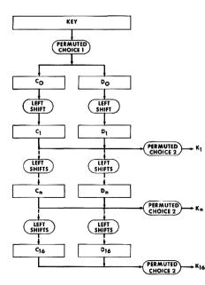
The key schedule of DES breaks the key into two 28-bit halves, which are left shifted by two bits in most rounds (only one bit in round 1,2,9,16) before 48bit are selected as the subkey for each round.
