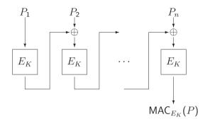
A modification of CBC provides integrity protection for data. The initial vector is set to a fixed value (e.g., 0), and  $C_n$  of the CBC calculation is attached to the transmitted plaintext. Anyone who shares the secret key K with the sender can recalculate the MAC over the received message and compare the result. A MAC is the cryptographically secure equivalent of a checksum, which only those who know K can generate and verify.
