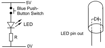
When the LED is lit correctly, the voltage across it will be about 1.6V and the current flowing through it should be about 15mA. To work out the appropriate value for R we need to use Ohm's law, i.e., V = IR. In this case the voltage across R is (5 - 1.6)V, so,
