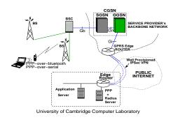
Fig. 2. The experimental testbed used for conducting the GPRS tests. A well provisioned, low latency tunnel transfers all Computer Laboratory GPRS device traffic directly to our PPP server.
