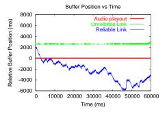
Fig. 6. The challenge of trying to maintain a sufficient buffer in advance of the media playout over a reliable GPRS link compared to transmitting data over an unreliable link.
