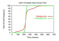
Fig. 3. The inter-arrival time CDF of packets (1000 packet samples, 1371 bytes size) with ARQ enabled and ARQ disabled.
