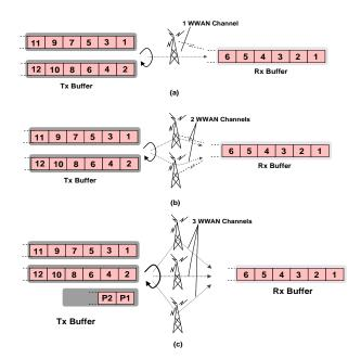
Fig. 13. The effects of interleaving over (a) 1 channel, (b) 2 channels and (c) 2 channels + 1 parity channel
