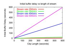
Fig. 7. The initial buffer delay that should be inserted prior to media playout in order to support various streaming rates.
