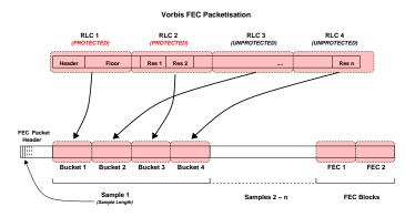
Fig. 12. The packetisation approach for utilising intra-packet error checking, and generating Unequal Error Protection for media such as Ogg Vorbis encoding.
