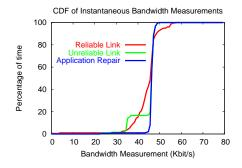
Fig. 5. The CDF of the measured capacity of the link, demonstrating unreliable, reliable and application repaired measurements.
