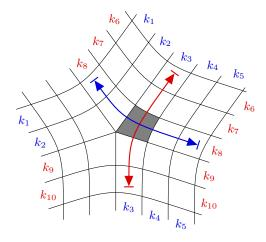
**Figure 5:** Every face has a local knot vector in two directions, which we can construct by following a strip of quadrilateral faces. For the shaded face, knot spacings in the blue direction are  $\{k_1, k_2, k_3, k_4, k_5\}$  and in the red direction are  $\{k_6, k_7, k_8, k_9, k_{10}\}$ . This example collects knot vectors at the length required for subdivision at degree 5.
