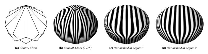
**Figure 12:** *Reflection lines on surfaces defined by a control mesh with a 12-valent extraordinary point. Each surface is rendered with vertices projected to the limit surface;* (c) *and* (d) *use exact evaluation [Stam 1998] to sample the limit surface in the region of the 12-valent point.*
