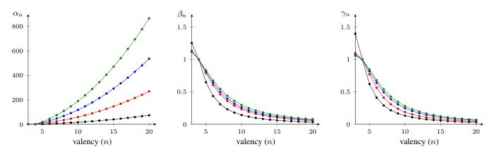
**Figure 9:** Bounded curvature solutions for  $\alpha_n^d$ ,  $\beta_n^d$  and  $\gamma_n^d$ . Valency ranges from 3 to 20. The multipliers are plotted for degree, d, equal to 3 -, 5 -, 7 - and 9 -. Note that  $\alpha_4^d = \beta_4^d = \gamma_4^d = 1$  by definition, as the regular case is curvature continuous and hence already satisfies the bounded curvature equations  $\lambda^2 = \mu_0 = \mu_2$ .
