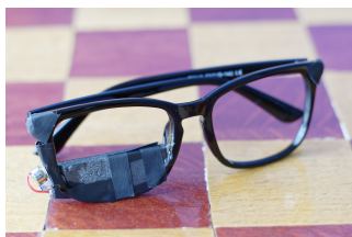
Fig. 6. Frames of the glasses with an IR LED. The participants were asked to wear these frames to track their head position.
