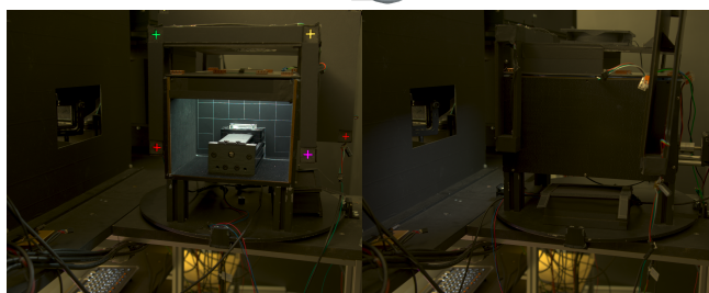
Fig. 7. The front and side view of the real-scene box and schematic of the calibration target inside. The calibration target has a grid of four-by-six squares of the size 30 mm \times 30 mm, which defines a world coordinate system. The red, green, and blue arrows in the figure represent the origin and orientations of the X, Y, and Z axes, respectively. We define the upper-left corner of the grid as the origin for the X and Y axes and the target placed at the front location as the Z = 0 plane.
