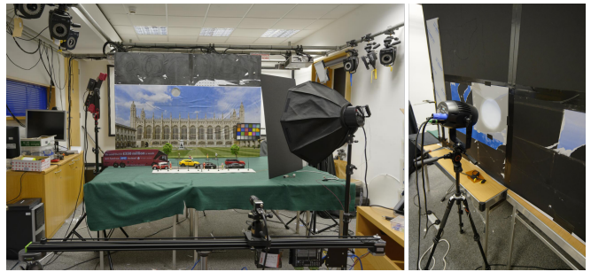
FIG. 1: The Street scene along with the capture and setup. Controllable lights are present on either side of the scene to simulate various lighting conditions. The right image shows the spotlight behind the scene, which shines through the diffuser and serves as a source of glare.
