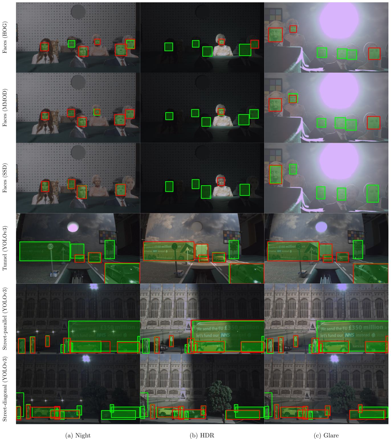
FIG. 5: Bounding boxes for several face and object detection methods (rows) for three adversarial illumination conditions (columns), each \gamma encoded (with \gamma = 2.2 ). Faces and objects detected by the various methods for the reference uniform illumination condition are shown as shaded green rectangles, while the results of the tested methods for other illumination conditions are shown as red rectangles. The text above each box shows the labels assigned by the detector.
