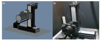
Fig. 1. CAD model of the light field capture rig (a) and its photograph (b).
