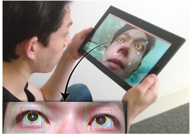
Figure 1: EyeTab enables gaze-based interaction with unmodified tablet computers in near realtime using a model-based approach for binocular gaze estimation.
