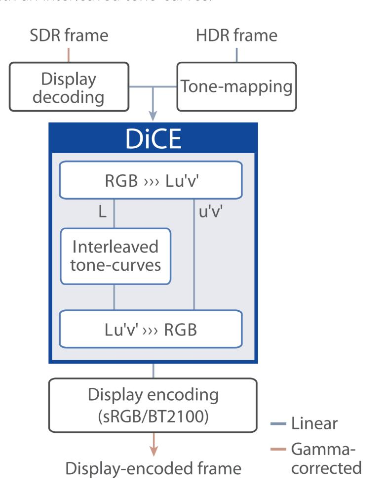
DiCE as part of a tone-mapping pipeline can take both HDR and SDR frames as inputs.
