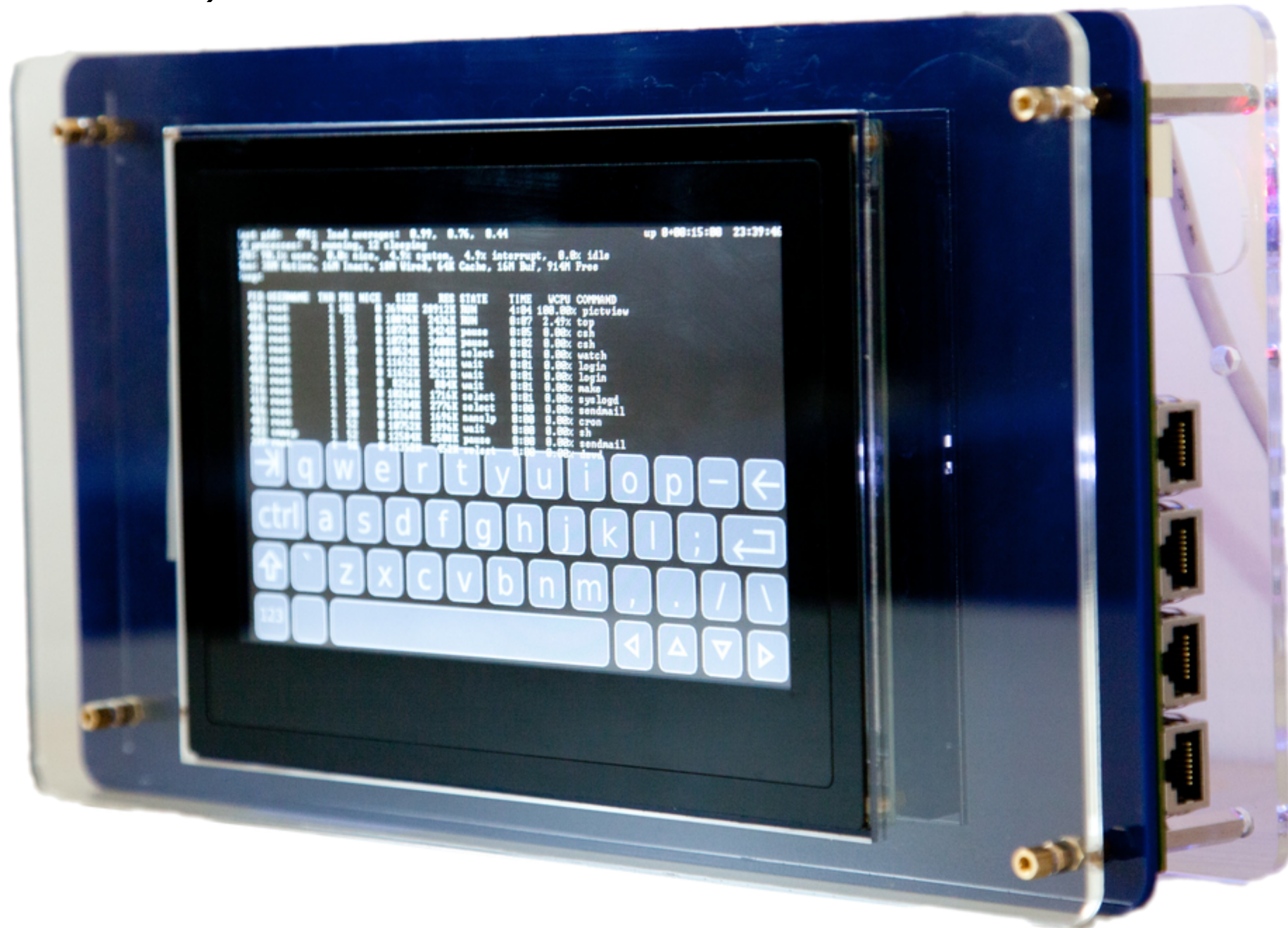
Figure 1: FreeBSD running on BERI on DE4 board
